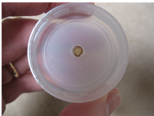
Aquarium tubing press-fit into drilled hole in bottle cap.
